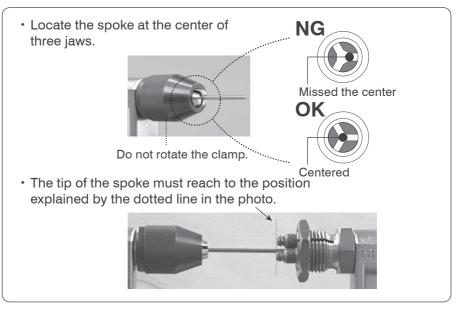
5 Slide the handle slightly toward the spoke so that the tip of spoke contacts with the center of three rollers of the die head.
